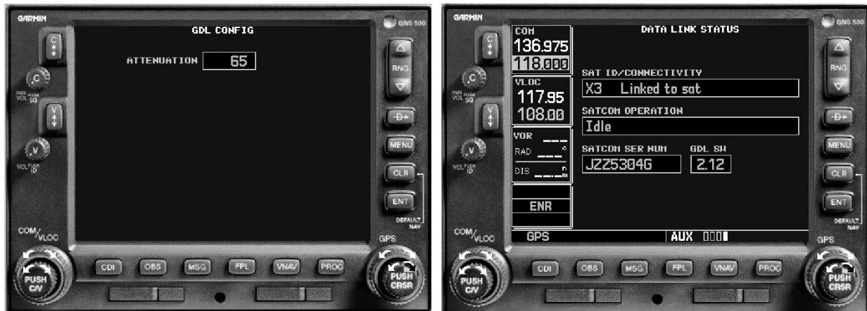
Figure 4-2. Data Link Configuration Page on the 400/500 Series (500 Series shown, 400 Series screen is similar)
